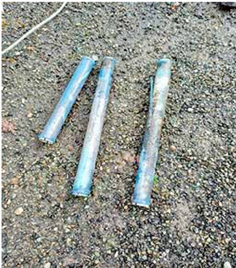
The aeration diffusers were damaged from silt and grit accumulation at the bottom of the treatment chambers. Their role is to deliver dissolved oxygen to the aerobic bugs that break down the wastewater organic matter.
